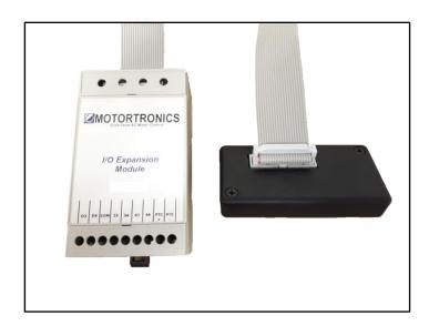
The adaptor module then connects to the VMX-agility<sup>TM</sup> edge connector as shown below:
