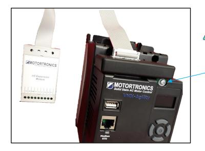
Fit screw and nylon washer (supplied). DO NOT overtighten (Max 40 cNm)
