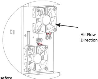
VMX-SGY-301 to VMX-SGY-305 have metal fan guards fitted for safety reasons. These must be removed before the fans can be taken off.
