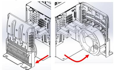
**4.** Remove the case moulding completely from the unit.
