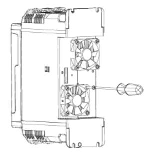
The recommended Part numbers for the replacement fans are detailed in the table below:
