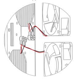
**8.** Fix the new fan(s) to the unit using the screws removed in step 1.
