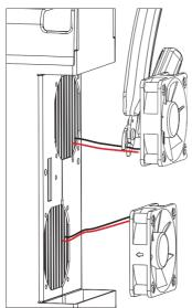
**3.** Fit the black wires from the new fan and the VMX-Synergy into the supplied connector.
