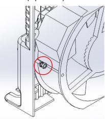
2. Slide the lower case moulding off the busbars and rotate it to the right. Ensure care is take not to damage the fan cable.
