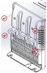
**3.** Disconnect the fan wires from the PCB terminal block. Feed the wires back through the fan wire hole.
