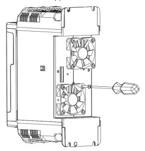
**2.** Cut the wires as close to the fan(s) as possible.
